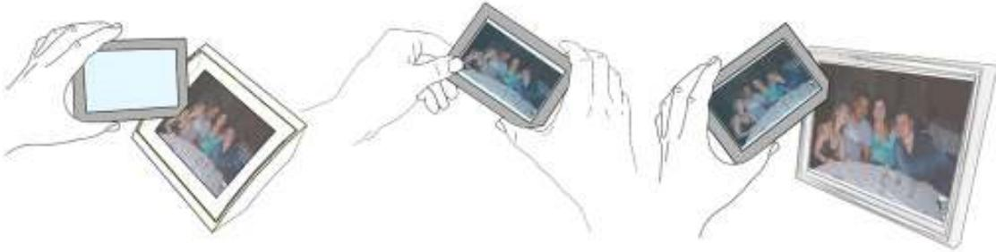
**Fig. 7 The Framer device – part of the initial Memories concept - was a small device used to transfer images between compatible surfaces. John Vines, 2006**
